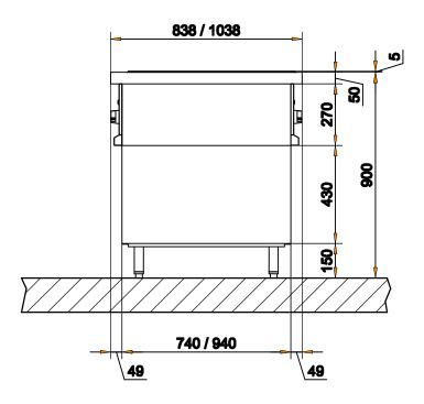
General Measurements - Room assembly of block - different base cainet depths possible
